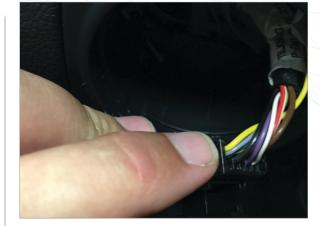
**OPTIONAL:** Connecting the dimmer line. The yellow wire for dimmer connection can be connected to interior illumination. Lighted vent wheels, LED backlights, pin 10 on most VW/Audi headlight switches, and on most BMW vehicles there is a red/gray wire many places, like the trunk pop switch.
