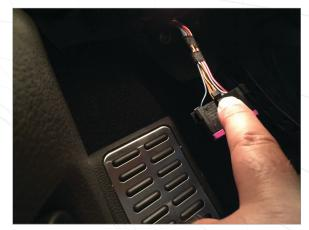
POWER CONNECTION: The gauge functions with a constant or switched 12v power source. The intellegent power sensing logic has no need for seperate constant and swtiched power sources, but rather tap any 12v power. A universal wire tap location for constant 12v would be pin 16 (BATT) and pin 4 (GND) on the obd2 port. The sleep batt check feature requires constant power.
