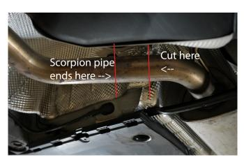
Line the resonator delete pipe up with the original exhaust and mark where the Scorpion pipe ends on the original.
