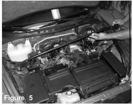
Figure 5 All four 12mm nuts have been removed and the strut tower bar is now pulled out.
