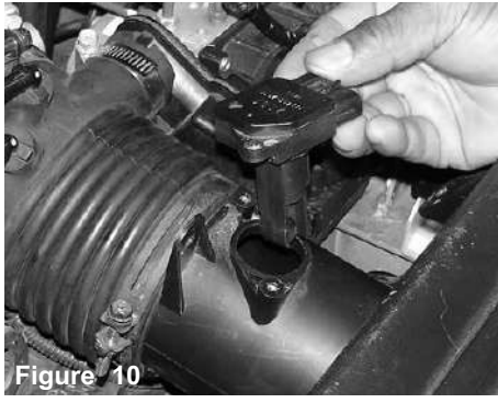
Figure 10 Once both screws have been removed, continue to pull the mass air flow sensor from the sensor housing.
