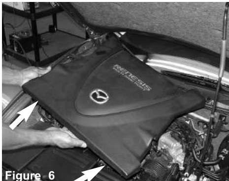
Figure 6 pull up on the stand offs located in front of the engine cover. A slight tug up will be required to pull the stand offs out of the stock grommet.
