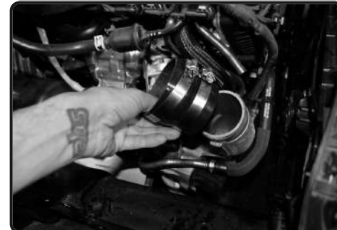
10. Install the provided step hose with clamps provided to turbo.
