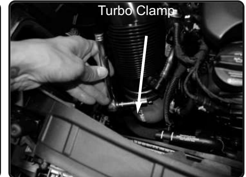
7. Loosen the clamp on the turbo using 7mm socket with ratchet.
