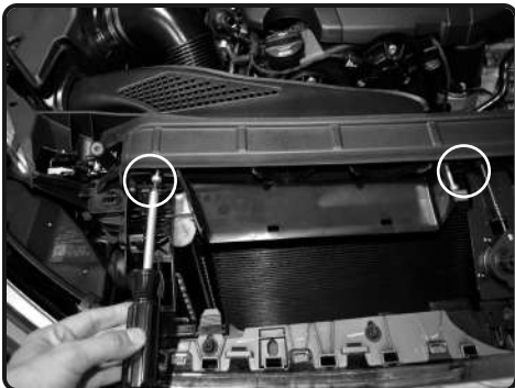
4. Locate the 2 bolts holding in the front air scoop and loosen and remove using T25 torx bit. Remove the 2 bolts.
