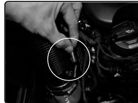
6. Pull back the vacuum line from the OEM intake tube.
