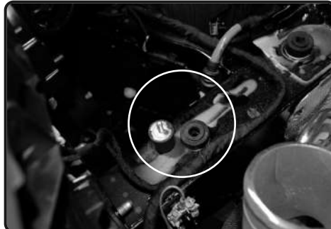
9. Now install the provided female/male M6 vibramount to the threaded stud on vehicle frame. Secure and tighten.
