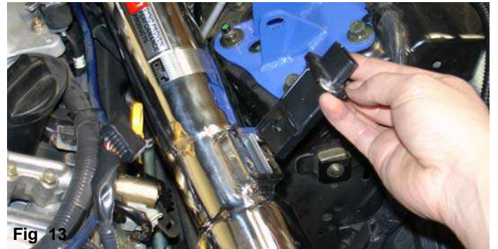
Fig 13 Press the stock MAF sensor into the machined adapter welded to the intake and use the stock screws to secure the sensor in place.
