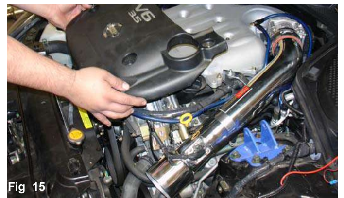
Fig 15 Once the entire intake is aligned and secured in place the intake manifold cover is re-attached.
