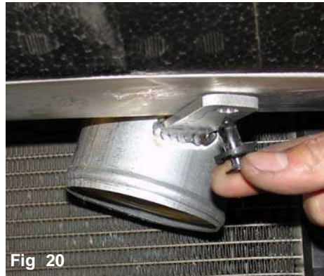
Fig 20 Line up the pre-tapped hole on the bumper reinforcement to the intake bracket. Use the stock plastic clip to secure the intake in place.
