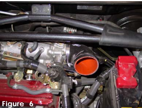
Figure 3 Remove the stock air intake duct connected at the throttle body (A) and the air intake box (B).
