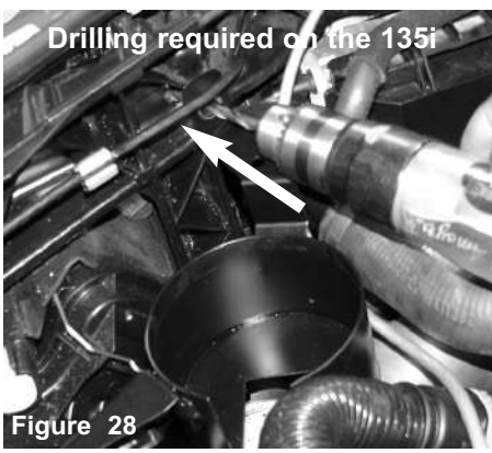
Figure 28 Applicable to the 135i only: Use a 1/4" drill bit to drill a hole through the composite cross member, the short bracket on the cup is used as a pattern.
