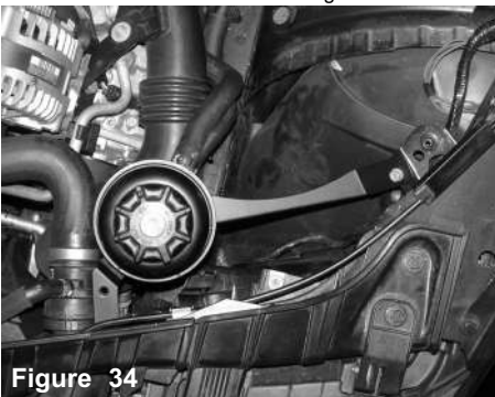
Figure 34 Install the reservoir into the cup and secure. Note: Make sure the reservoir bottle sits all the way down and tight.
