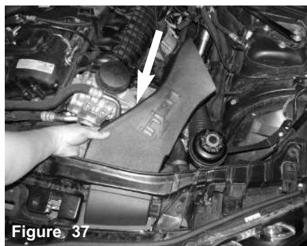
Figure 37 Install the driver side factory scoop, position the Injen power-scoop to the back of the core support, locate the 2 inserts through the scoop. Secure the power-scoop using the 2 remaining M6 button head screws.
