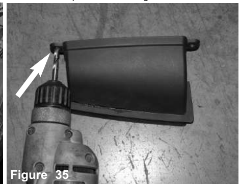
Figure 35 Drill all the 4 holes out to 1/4" on the factory scoops to make the M6 screws able to pass through.
