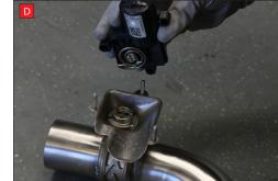
A) After you have removed O.E exhaust you will need to swap the valve motor to the Scorpion exhaust. Remove the 3 nuts (keep them safe, as you will need them to bolt the electronic valve motor to your Scorpion Exhaust).
