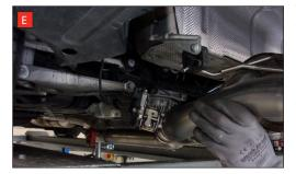
The valve motors on the original system are required when fitting the Scorpion system.
