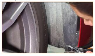
09. Pull back on the fender liner to access and remove the bolt that secures the corner of the bumper to the fender. Do this on both sides. (2x 8mm bolts)
