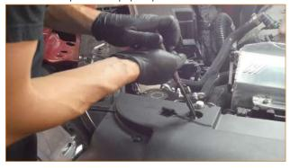
Remove the six screws that secure the top edge of the bumper. (6x 8mm screws)
