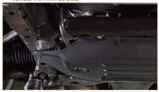
**05.** Locate the radiator drain on the passenger side of the vehicle. Install a short piece of hose over the drain to avoid spilling coolant. Place a drain bucket under the hose, and loosen the drain plug until coolant flows freely from the hose.
