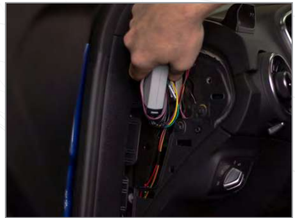
12 Tuck control box and wires into side dash
