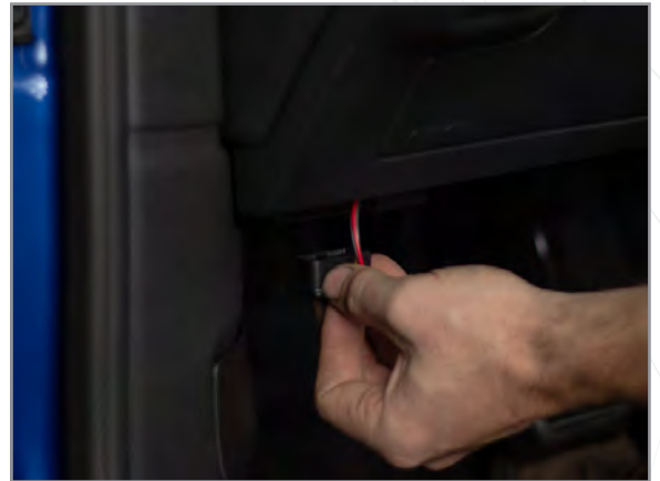
14 Plug the OBD2 cable into the vehicle's OBD2 port
