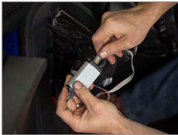
11 Connect both the display cable and the main harness to the control box
