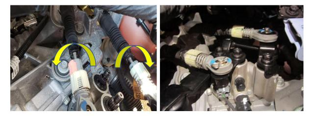
**11**. Tighten the three fasteners that hold the linkage to the gearbox, then test to see how the shift feels inside the car. If you think it needs adjustment this is the time to do so, now reassemble by following the steps 1-6 in reverse.
