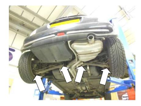
2. Using a suitable penetrating oil lubricate the threads on the bolts at each end of both tie-bars. Wire-brush the threads if necessary to remove any excess debris.
