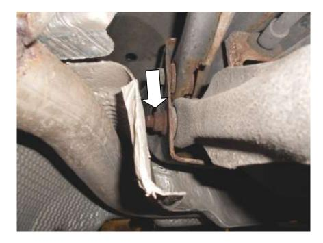
6. Using a paint marker, centre dot or cold chisel mark the position of the snail cam adjuster.
