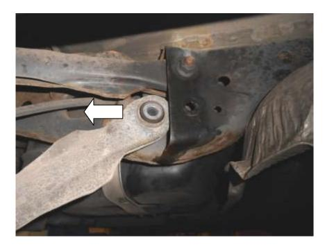
11. Using the standard tie-bar and OEM bolts match the bolt hole centres on your Forge adjustable tie-bars. This is just to set a baseline you will need to get the tracking checked after the installation is completed. Using a pair of adjustable spanners lock both locking nuts when the tie-bars are set at the correct length.
