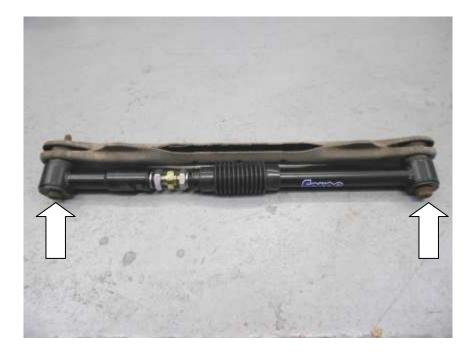
12. Install your Forge tie-bar in the reverse of the disassembly. The short side of the tie bar fits closest to the wheel hub.
