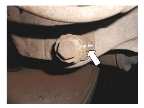
7. Using an 18mm socket, short extension bar, suitable ratchet and 18mm spanner undo the top bolt and remove it. Access is very restricted to get the 18mm socket on the head of the bolt.
