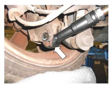
15. Re-install the snail cam adjuster and bolt.
