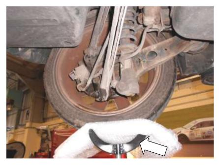
4. Undo the 1x 8mm screw, 2x 10mm bolts, and 2x 10mm nuts. Pull the exhaust heat shield towards the back of the car and downwards to release it. Let the heat shield rest on top of the exhaust, it does not need to be fully removed.
