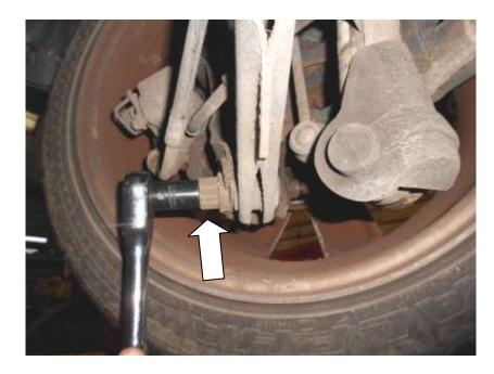
9. Place a piece of packing material between the lower part of the tie bar and the wheel. Pull the tie-bar downwards to release it.
