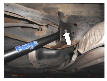
13. Insert the chassis end first and replace the nut and bolt. Do not fully tighten.
