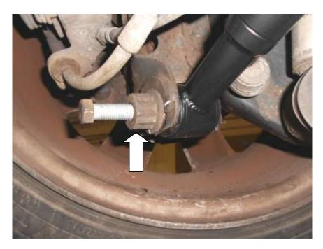
16. Using 24mm Ring-spanner rotate the snail cam adjuster into the position marked during disassembly. Using a 16mm socket and 1/2" ratchet tighten the centre bolt and lock the adjuster in position.
