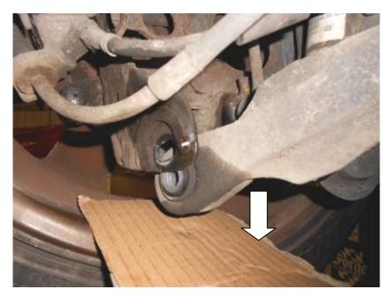
10. Pull the tie-bar towards the outside of the vehicle at the top to release it.
