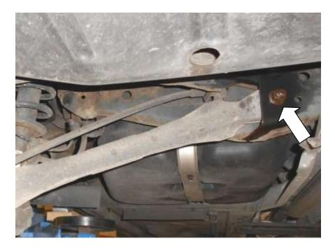
8. Using a 16mm socket and suitable ratchet, undo the lower bolt. Carefully remove the snail adjuster and bolt. Keep Left-hand and Right-hand snail adjusters separate if both tie-bars are being removed at the same time.
