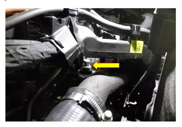
**12**. Using a 8mm socket and ratchet or flat bladed screw driver loosen off the two hose clamps securing the rubber boost hose in situ and remove the hose from the engine bay.
