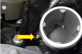
8. <u>IMPORTANT</u> Make sure not to lose the O-ring when removing the turbo elbow.
