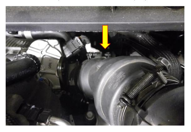
4. Slide the grey locking tab back to allow you to disconnect the loom attached to the turbo actuator.
