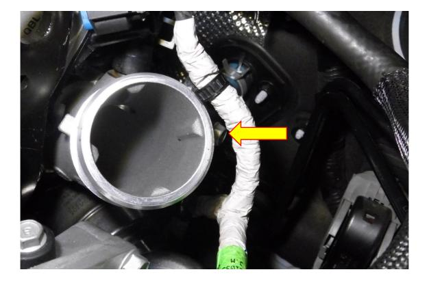
6. Using long nose pliers loosen the hose clamp to allow the removal of the oil breather pipe attached to the turbo adaptor.
