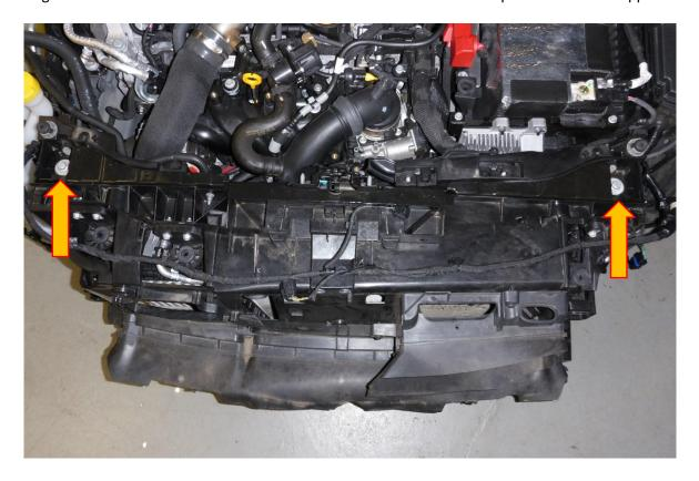
15. Remove the X2 fasteners at the bottom of the radiator support frame. There is one on each side. The radiator frame will now lift upwards and then away, it will still be attached via the bonnet release cable however there is enough slack to allow it to be positioned out the way.
