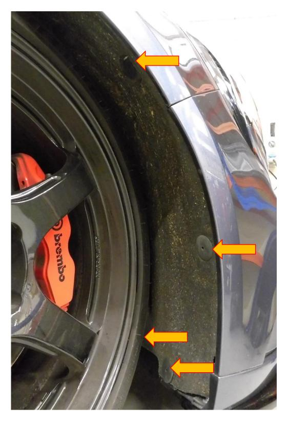
4. Peel back the arch liner so you can gain access to the 10mm fastener attaching the corner of the bumper to the wing. Using a 10mm socket and ratchet remove both fasteners X1 each side. With a sharp pull of the bumper this will release it from the wing.
