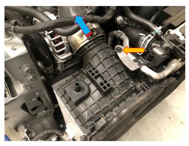
17. Un-clip and remove the bottom boost pipe from the intercooler.
