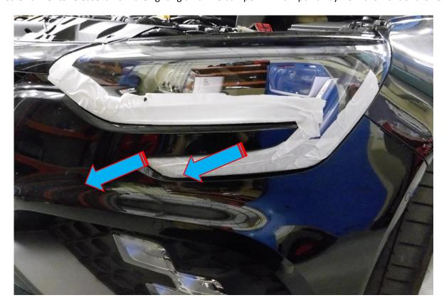
8. Un-plug all three connectors and unclip the loom at the rear of each lighting unit.
