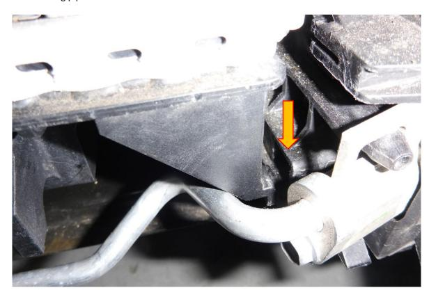
20. Place the Forge Motorsport intercooler in place, make sure the bottom mounting peg is located into the rubber grommet. Attach the lower boost pipe, push it all the way on until you hear a positive click.
