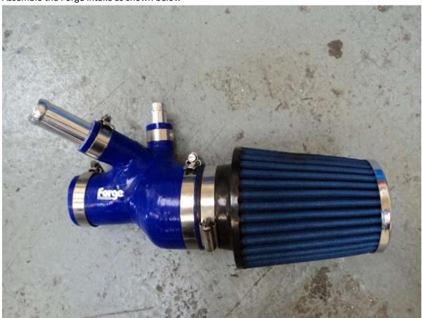
12. Place the intake on the turbo and orientate it so that the pipes on the car line up with the pipes on the intake, then tighten the hose clamp on the turbo, and oil breather lines.
