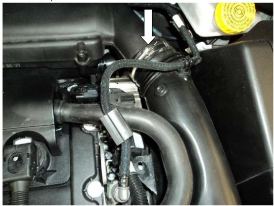
2. Remove the clip holding the breather to the inlet pipe and remove the pipe, remove the moisture sensor wiring, and remove the feed to the brake master cylinder by depressing the green push in section and lifting the hose upwards.
