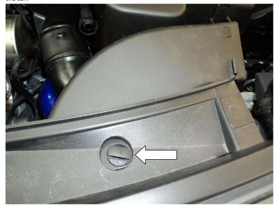
5. Remove the clip holding the cold air feed to the rear of the slam panel and unclip the pipe from the battery tray so the end is free.
