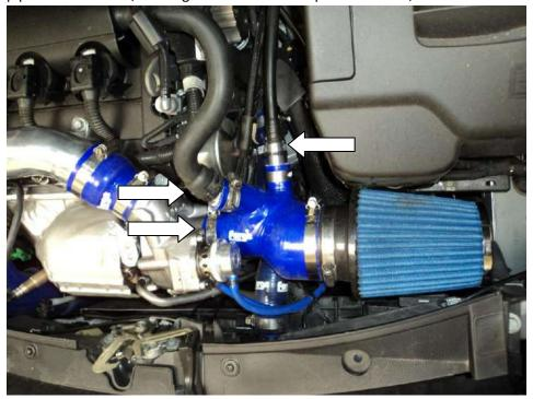
13. The intake installation is finished. You'll notice that the intake now sits right behind the cold air feed which results in much cooler inlet temperatures.
