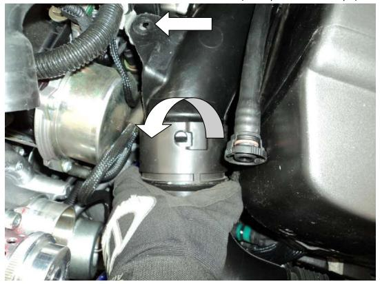
7. Rotate the last pipe clockwise out of the bottom of the intake (its held on a rubber o-ring) to release it, then remove it from the car.
