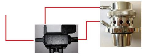
11. Once you have cut and run the silicon hose, secure each end with the supplied cable ties. Use the large able tie to tidy and secure the hose and wiring loom. Make sure the wiring loom to the solenoid is not stretched or bent over too sharply, it should look like the picture below.
