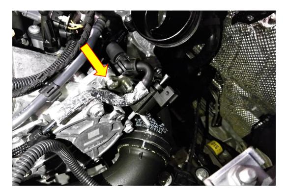
7. Take the wiring loom supplied in the kit and connect it to the solenoid and the other end to the loom which was attached to the OE valve.
