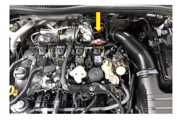
3. On the OE valve push back the red retaining clip to allow you to remove the wiring loom. Remove the three T30 Torx fasteners attaching the OE valve to the turbo, the OE valve will now come away from the turbo.
