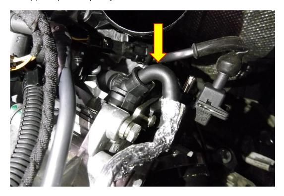
9. Using the supplied brass T piece and silicone pipe attach it to the vacuum pipe removed in the previous step just like it is in the picture below.
