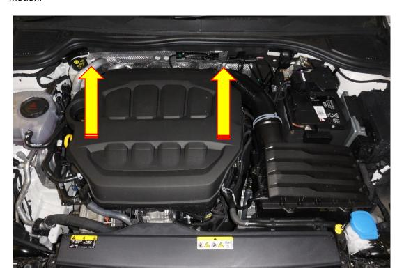
2. With the engine cover removed locate the original diverter valve.
