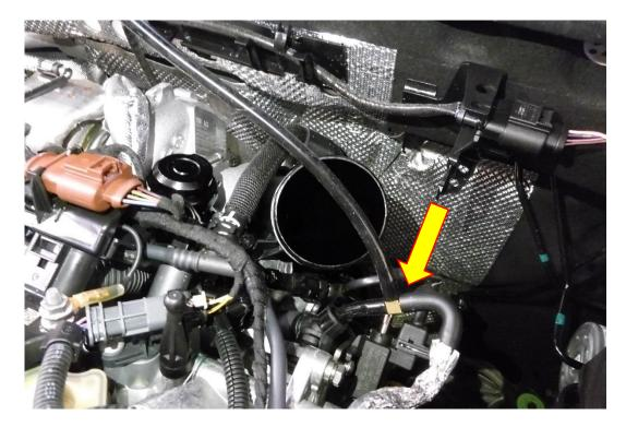
10. The next set of pictures are for illustration purposes - they may not be representative of your engine, but they are the clearest way to show you how to connect your solenoid to the atmospheric or recirculating valve you have fitted. Use the supplied silicone hose to do this, use a sharp knife or side cutters to cut the hose to length.
