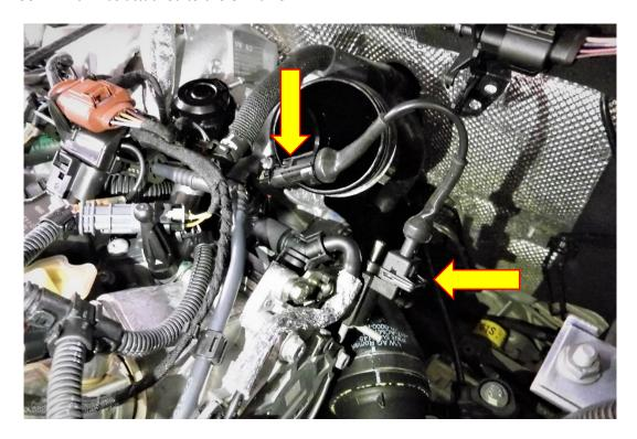
8. The vacuum source in the engine bay is next to where the solenoid has been fitted. Pull the vacuum pipe away from the plastic joiner.
