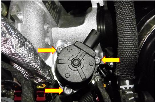
4. Take the Forge Motorsport valve and mount it into position where the OE valve used to be. Use the original T30 Torx fasteners to secure it in place.
