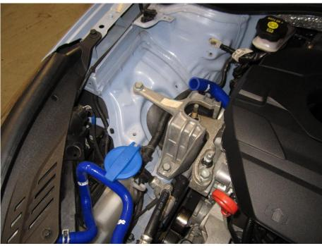
2. Remove the engine cover by pulling it upwards from both sides of the cover.
