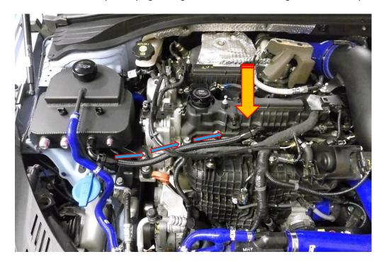
9. Attach the AN-6 fitting of the smaller hose to the catch tank and run the hose to the rocker cover as shown in the picture below. Use a 17mm spanner to tighten the AN-8 fitting and a 7mm socket to tighten the hose clamp on the breather end of the hose.
