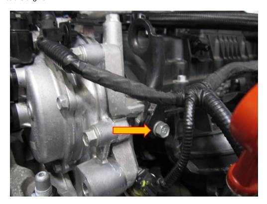
8. Fit the coolant return hose to the expansion tank. Attach the AN-8 fitting hose to the catch can use a 22mm spanner to tighten. The alloy fitting at the other end of the hose locates to the lower front oil breather. Once happy with the orientation of the hose tighten the boss and the AN fitting with a 22 & 26mm spanner and push the fitting into place. Finally secure the machined boss in place by tightening both M4 fasteners using a 3mm Allen key.
