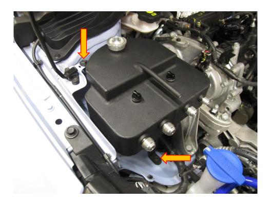
6. Take the AN-8 line and attach the machined boss with two the M4 fasteners to the 120 degrees end of the oil line, but only hand tight at this stage.
