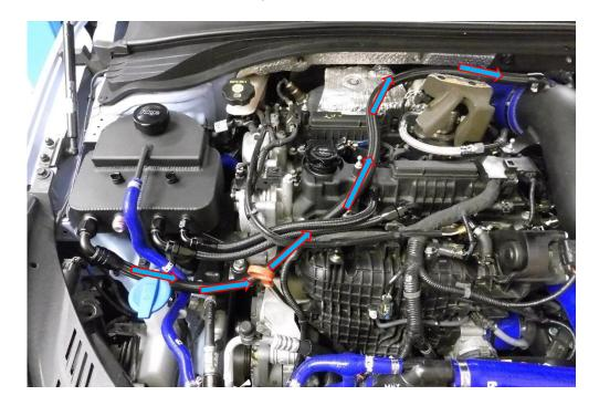
11. The last hose to be installed is another AN-10, run the hose as shown in the picture. As in step 8 the breather end has a push fit machined boss which is secured in place with a M4 fastener. Use 26mm spanners to tighten.
