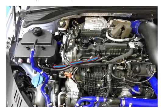
10. Take the longest hose from the kit and run the hose as shown in the picture below. Unclip the wiring loom to the injector behind the oil cap, this will allow you to run the hose underneath it, then re connect the loom. Use a 25mm spanner to tighten the AN-10 fitting and a 7mm socket for the hose clamp at the other end of the hose.
