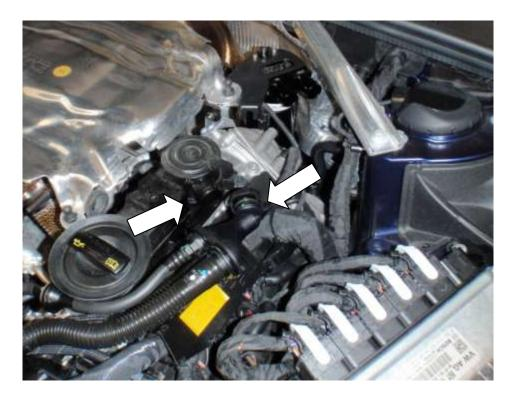
7. Use hose 1 to connect the cam cover breather outlet to the inlet side of the catchcan.
