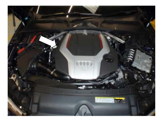
3. Using a 13mm spanner undo 4x engine cover mounts and remove the metal heat shield.
