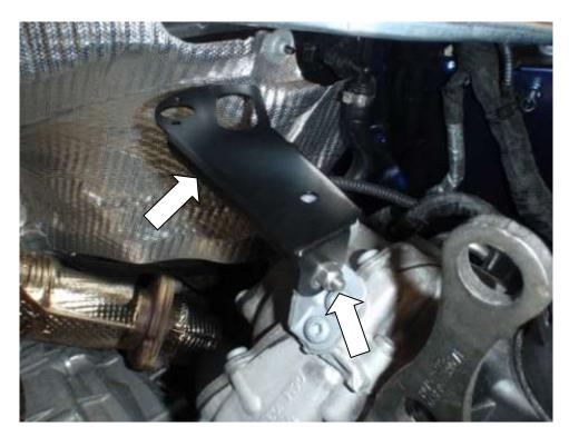
5. Using the 2x M4x8mm Allen cap bolts provided secure the catchcan in position. Ensure that the drain tap on the bottom of the catchcan is in the closed position.
