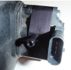
4. Fit the supplied hose to the nipple and route to the required location.
