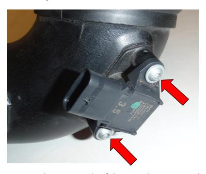
2. Insert the sensor into the correct side of the Forge boost tap as shown below.
