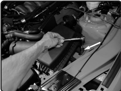
5. Remove the 10mm bolt from the OE air box assembly and then remove the entire OE air box assembly from the engine bay.
