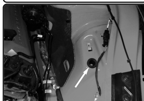
11. Install the larger grommet from figure 8 and install it into the original hole location on the fender well
