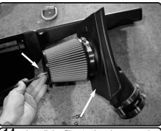
14. Install the filter to the plenum and tighten using 8mm nut driver. Connect the 3mm vacuum line from the filter minder to the barbed fitting on top of the filter.
