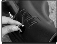
**3.** Install the plenum assembly into the air box. Secure using provided M6x20mm phillips screw with rubberized washer.
