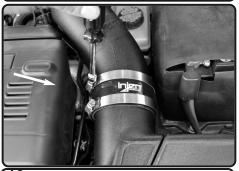
**10.** Tighten the hump hose using 8mm nut driver.
