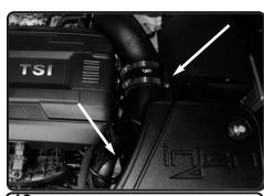
**12.** Now route the hose under the intake tube and connect to the 1/4" fitting.
