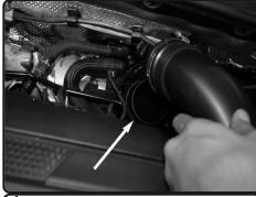
**4.** Pull back the intake tube from the turbo housing.
