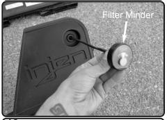
**12.** Attach the 3mm hose to the Filter minder and install the hose through the grommet.
