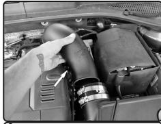
**8.** Install the intake tube to the vehicle. Position the tube to step hose and hump hose.
