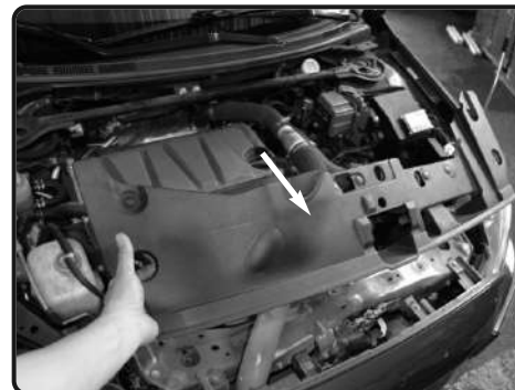
7. Remove the plastic retaining clips to remove the radiator support cover.
