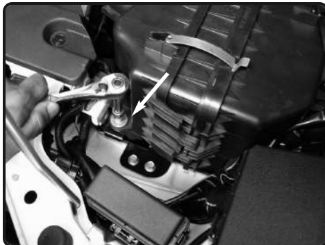
5. Remove the 10mm bolt from the Oe air box attached to the mounting bracket
