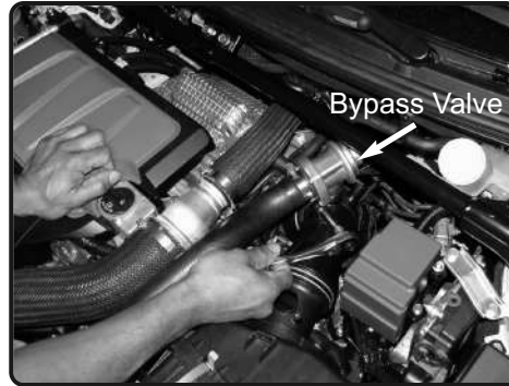
2. Loosen the clamp on the OE bypass valve. Detach the bypass valve from the stock air duct tube and place it to the side for now.
