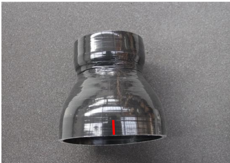
31. Mark the high point with a pen.
