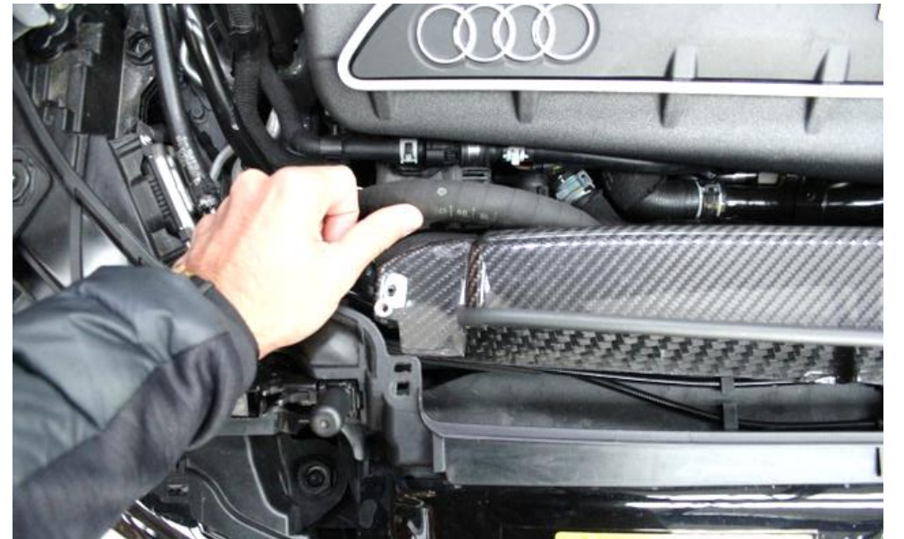
48. Push the engine hose forwards slightly to give the duct clearance to drop into position.
