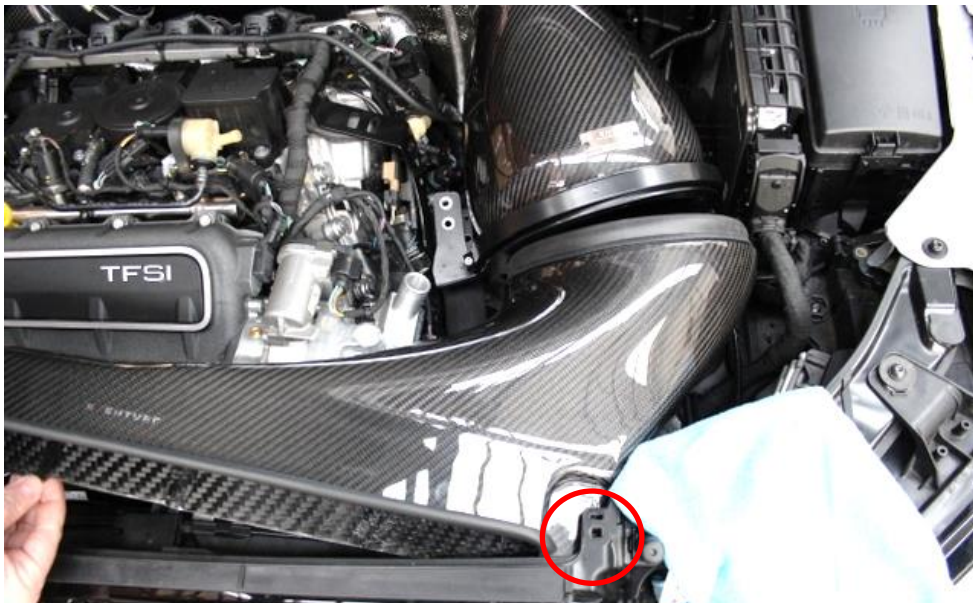
47. Now rotate the duct so the rear corner goes into the mounting location circled.
