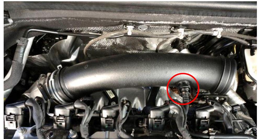
10. Remove the spring clamp holding the turbo tube to the rubber joiner and also the breather connector circled in red.
