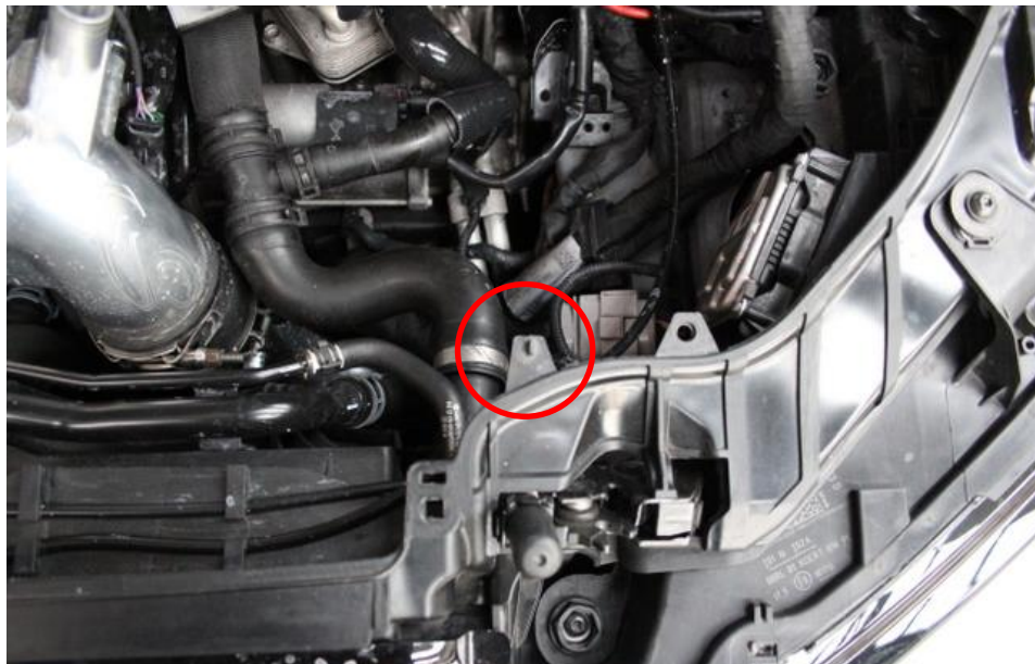
43. Before placing the duct – we need to cover this plastic tab with a cloth to prevent scratches.
