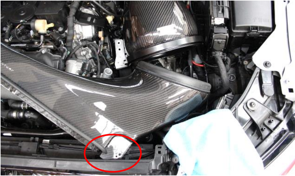
45. Carefully angle the duct down as shown. The rubber seal will touch the filter housing and the back edge should go inside the slam panel as circled. See next photo for another angle.
