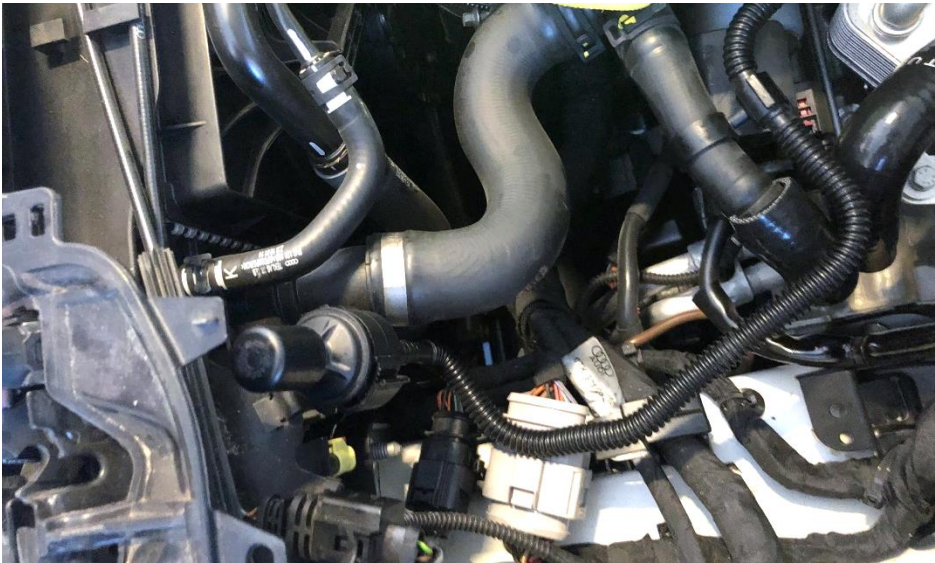
29. Route the Oil breather pot to the panel behind the headlamp – make sure the oil line is routed as shown
