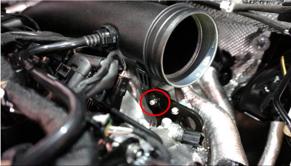
9. Remove the screw securing the Turbo Tube.
