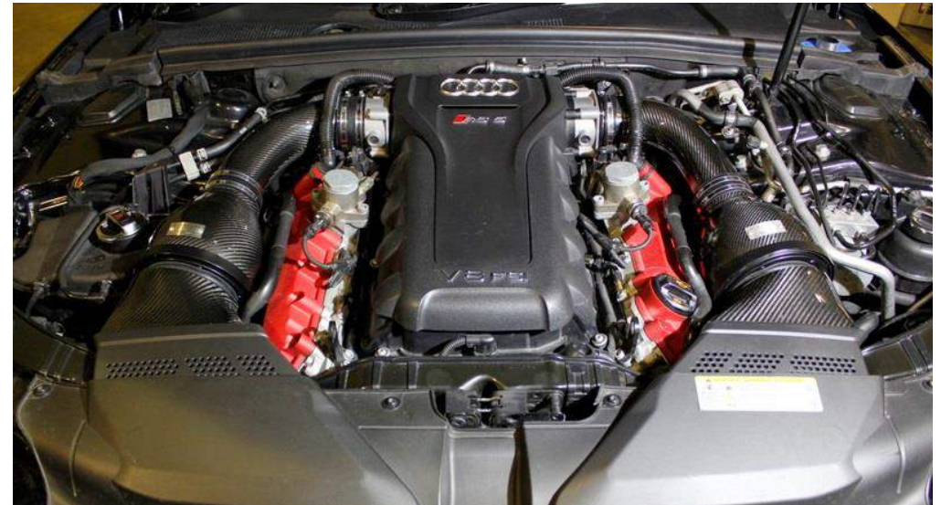
61. Reinstall the stock duct cover and ensure all hose clamps for the intakes are secure.
