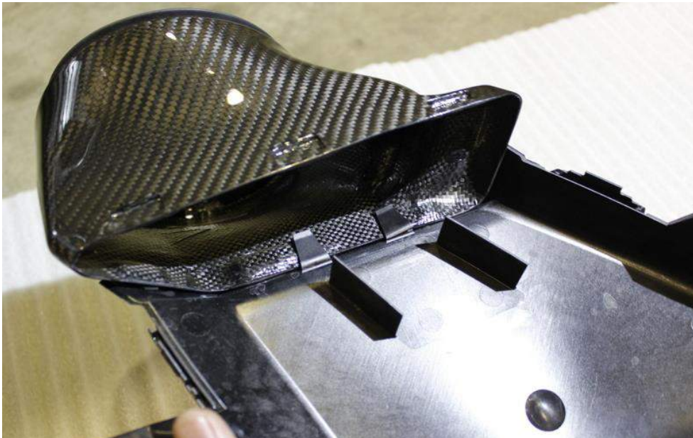
37. Take the LHS carbon duct and LHS stock plastic duct. Push the carbon duct into the plastic duct as shown.
