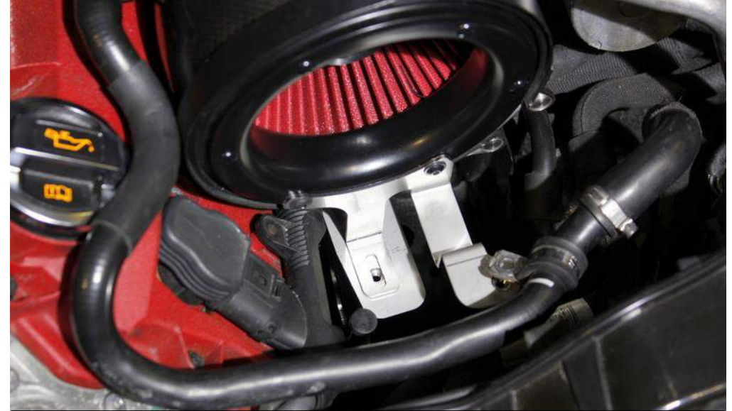
59. The bracket on the air hose should go on top of the housing bracket as shown.
