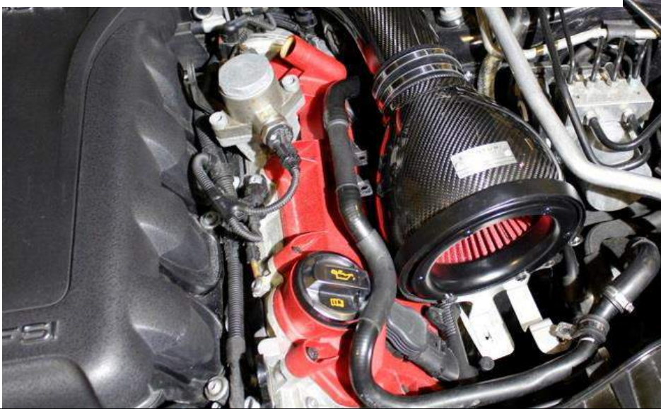
58. Push the RHS housing into place and lower the intake down to rest the bracket onto the heat shield. Lift the secondary air hose over the oil filler cap for more clearance.
