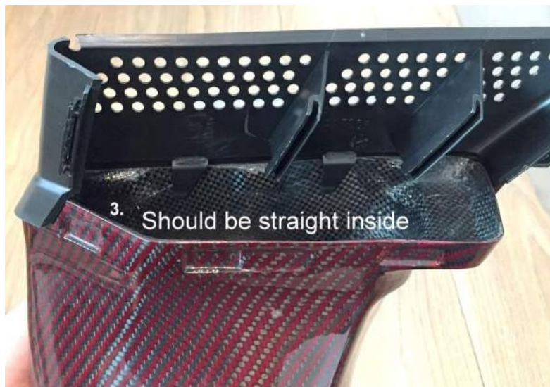
37. Take the LHS carbon duct and LHS stock plastic duct. Push the carbon duct into the plastic duct as shown.
