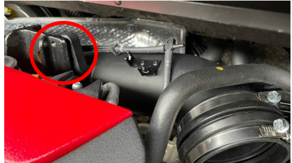
18. Insert the tube into the OEM rear rubber hose. Rotate the tube so that the tube mount lines up with the metal bracket. Do not insert the newly supplied 13mm bolt yet.
