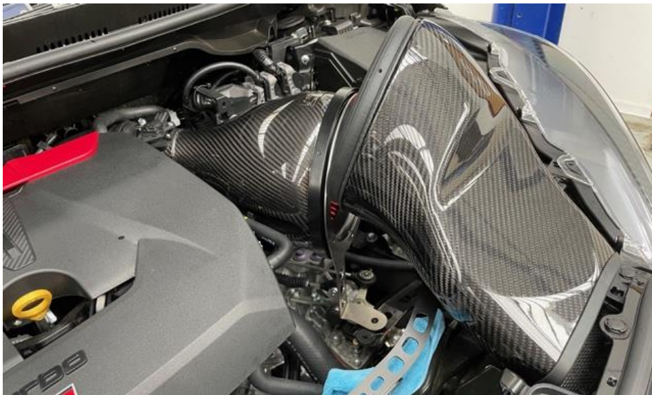
27. Carefully insert the duct – push the housing back to give enough clearance.
