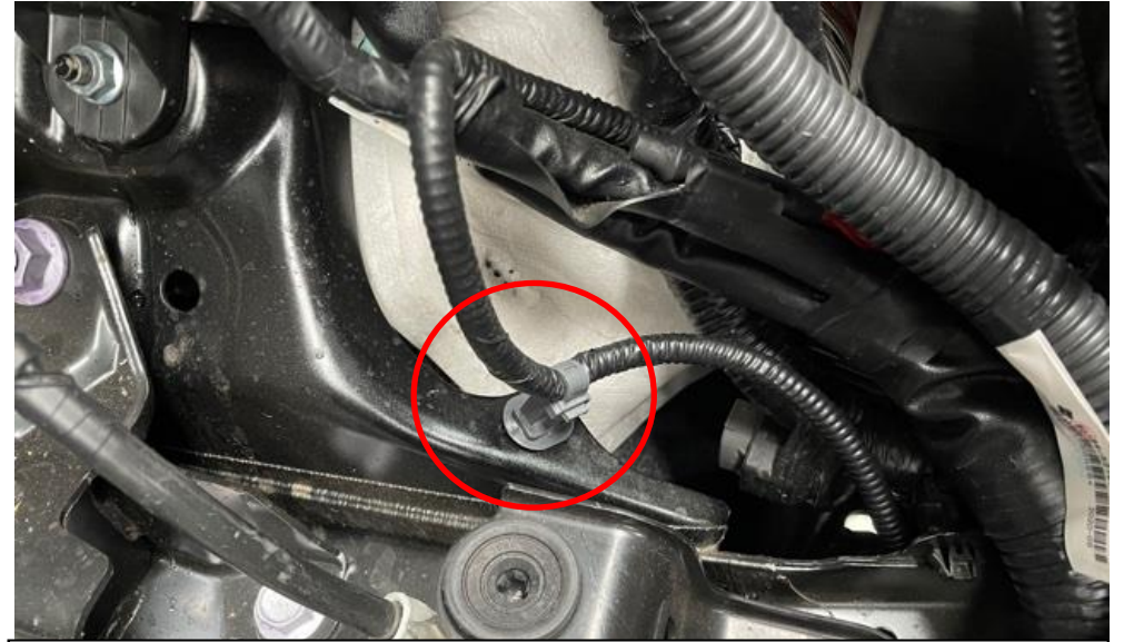
22. Clip the loose vacuum module plug into the spare hole on the chassis next to the airbox mount and tuck away the plug into the arch.
