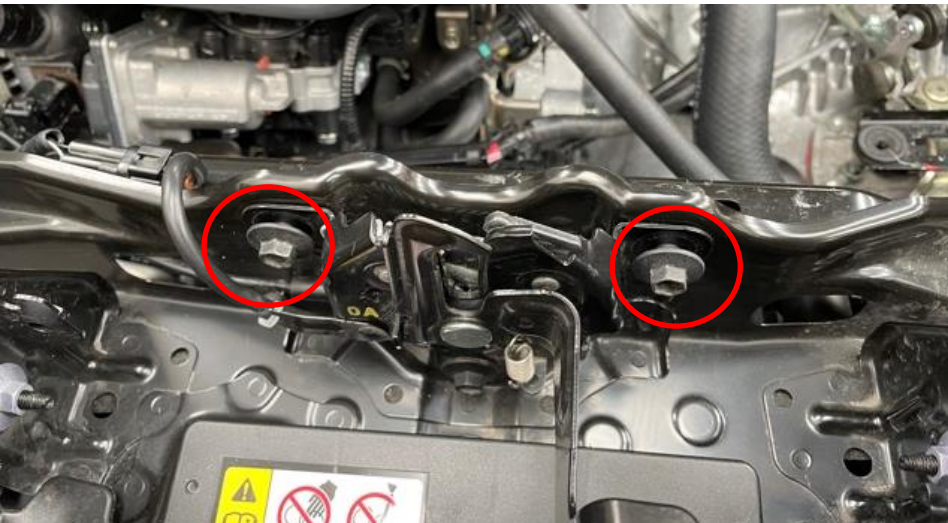
15. Remove the 2 M6 bolts from the sides of the bonnet catch. REPLACE them with the new M6 bolts supplied.
