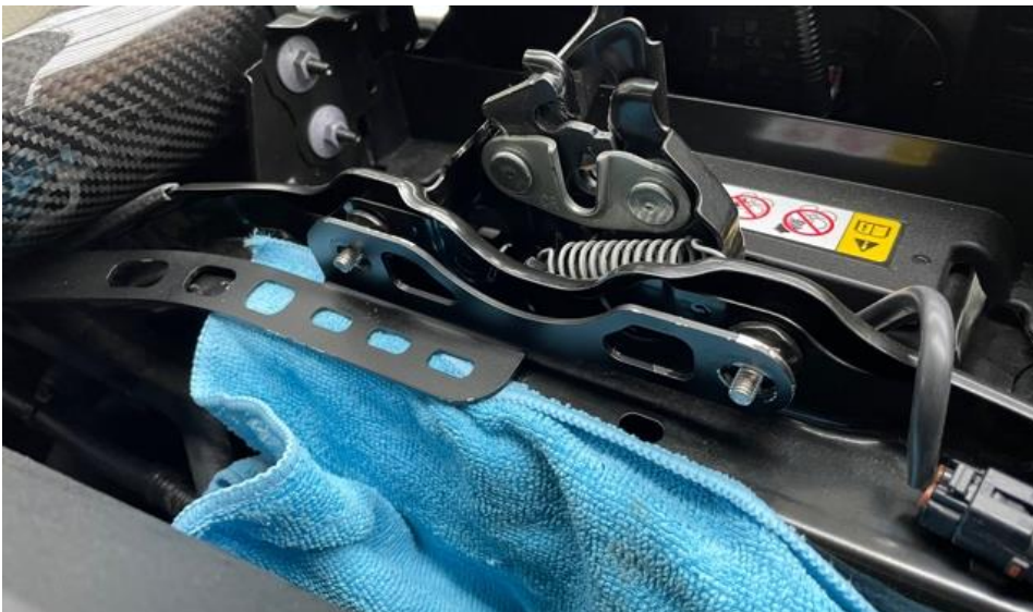
31. Position the lower bracket over the new M6 bolts installed previously. Remove the cloth.
