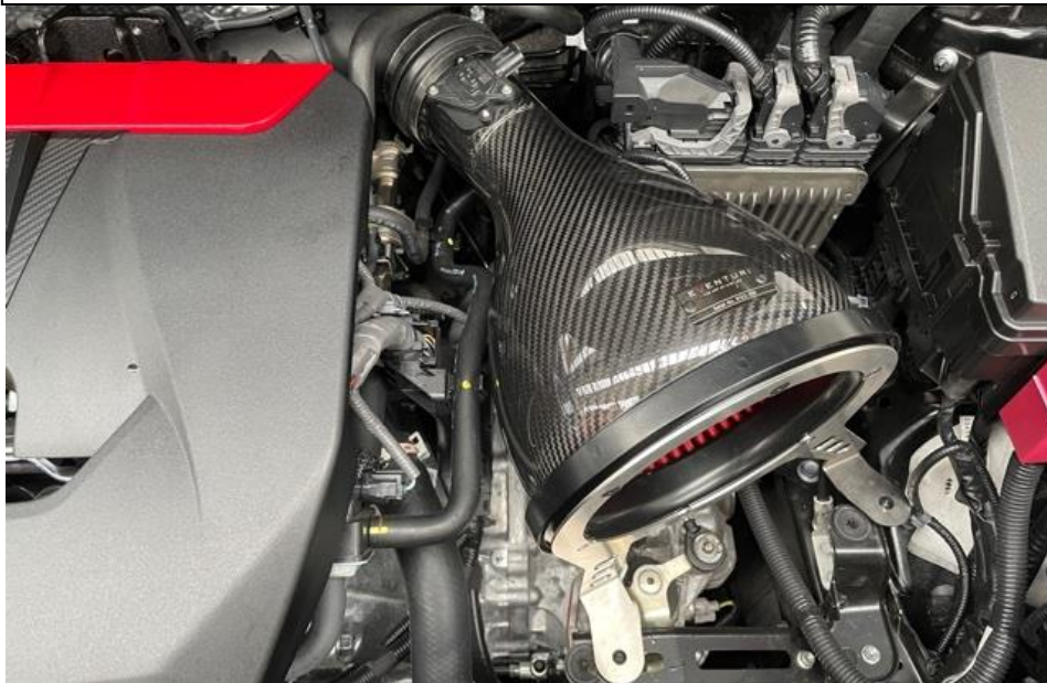
23. Insert the carbon housing into the flexible hose – DO NOT tighten it. Do not mount the feet to the rubber grommets yet.
