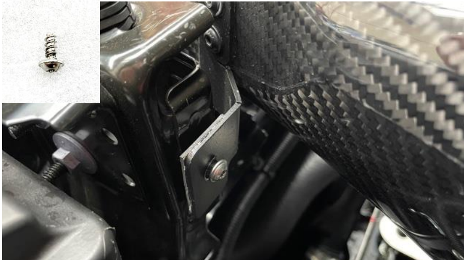
33. Using the supplied M5 cutting screw as shown - screw into the white clip through the bracket but DO NOT tighten yet.
