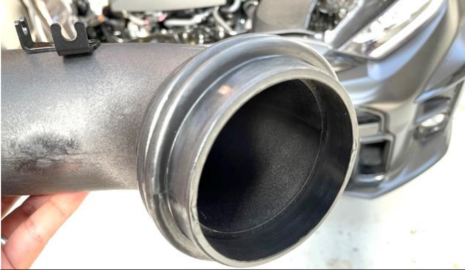
17. Push the hose all the way up to the last visible internal rib of the hose. It should look smooth on the inside like this. Tighten the hose clamp around the tube.
