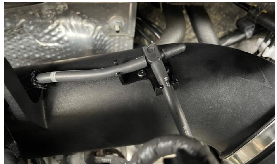
20. Plug the T-Piece with the supplied banking plug and secure it to the bracket on the tube.
