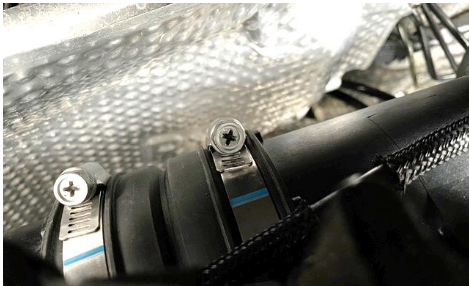
19. With the tube mount rotated into the correct place – tighten the hose clamp around the tube.
