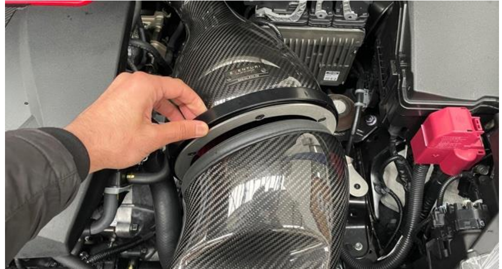
34. Now position the housing into the correct location and push the bracket mounts onto the rubber grommets – see next step.
