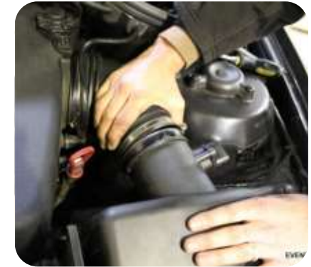
4. Loosen hose clamp and pull the airbox out of the elbow.
