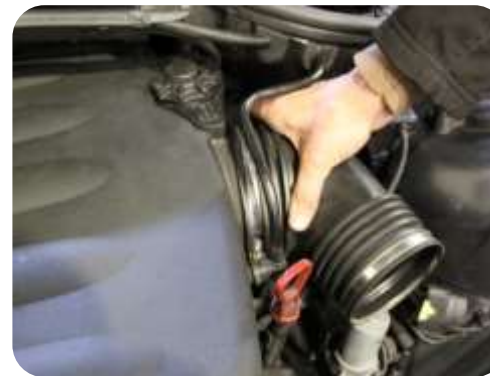
7. Loosen hose clamp for the elbow at the plenum end and rotate the elbow down slightly. Leave the hose clamp loose.
