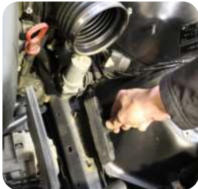
5. Remove Rubber mount from chassis by simply pulling off.
