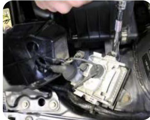
2. Remove Headlamp Module cover and remove the 2 bolts and 1 nut using 10mm socket. Once done, remove the module completely.
