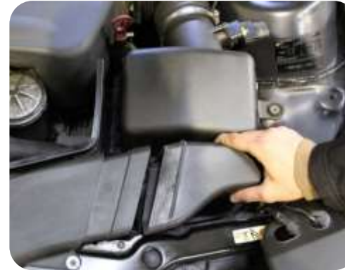
3. Remove extension duct by pulling away from the main part and then lifting up from the airbox.
