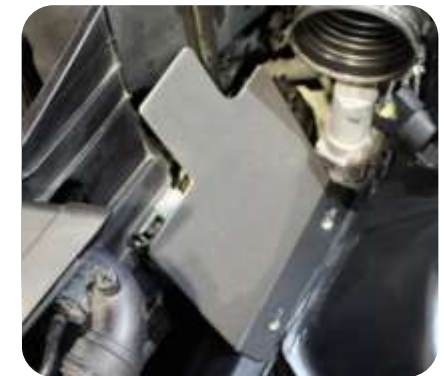
8. Install Secondary Heat Shield onto chassis by using the exposed studs revealed from step 5. Use the supplied flanged nuts to tighten.
