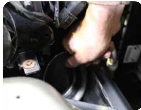
6. Remove Intake Tube connected to the brake duct (below headlamp) by pulling up. You may need to compress the part protruding into the brake duct.
