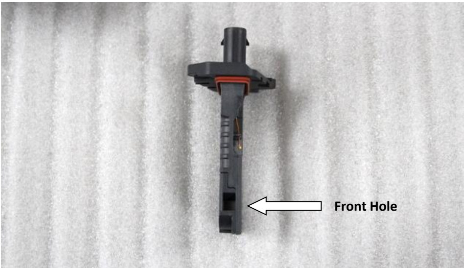
15. Remove the MAF sensor from the airbox. The front of the sensor has the hole as shown – this MUST face the filter when installing into the carbon tube in next step.
