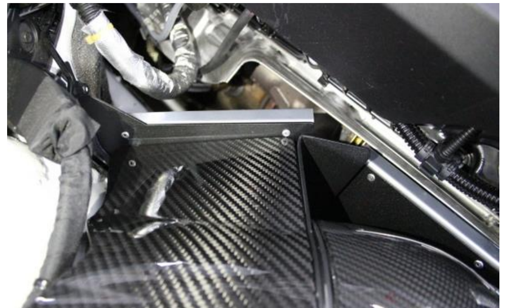
20. Rotate the carbon housing so that the carbon shroud lines up with the heat shield as shown.
