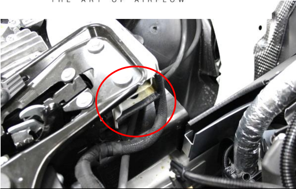
17. Push the supplied rubber strip over the corner of the bodywork as shown.
