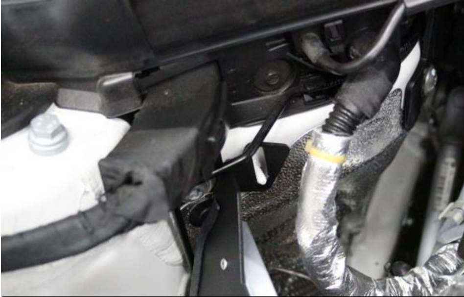
13. The top of the shield should locate into the upper threaded stud on the bodywork.
