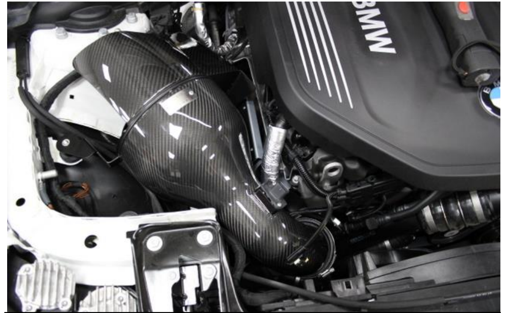
18. Carefully lower the intake into the engine bay and position the tube into the silicon coupler.
