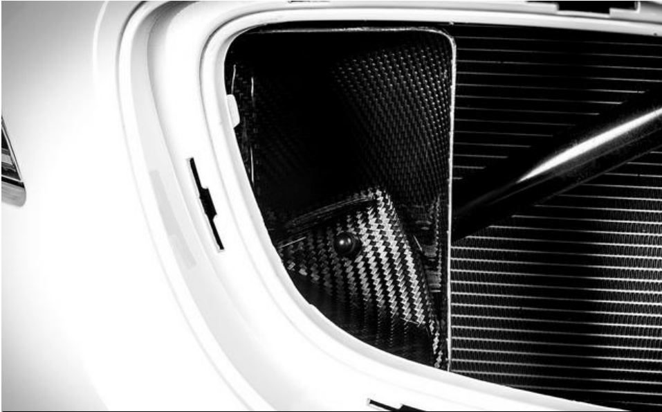
29. The scoop should sit as shown. The grill can now be pushed back into place.
