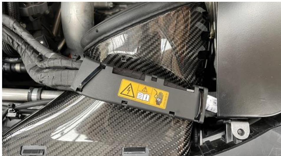
27. Using 2 zip ties, secure the cable cover removed in step 2 to the duct. Pass the zip ties through the holes in the top of the duct.
