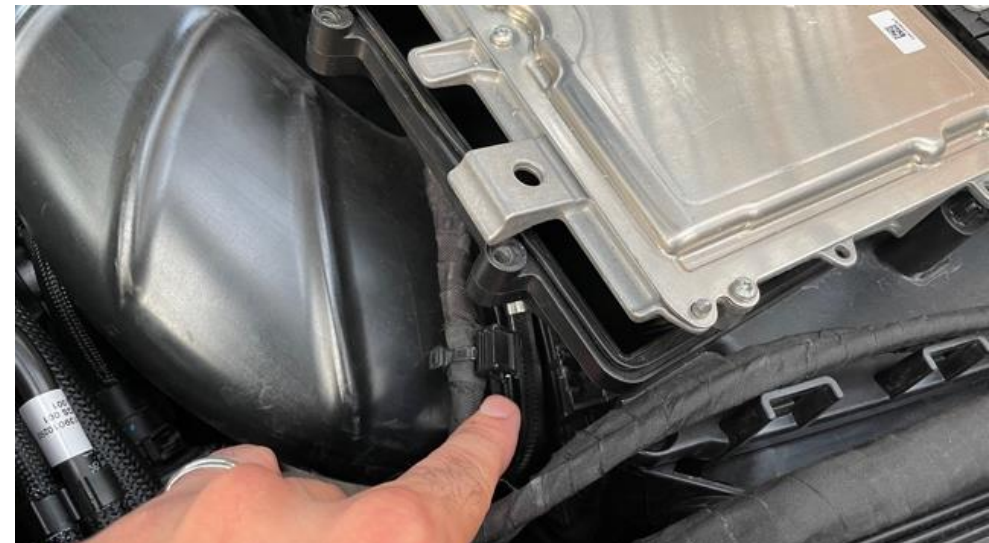
4. Unclip this wiring harness from the side of the airbox.
