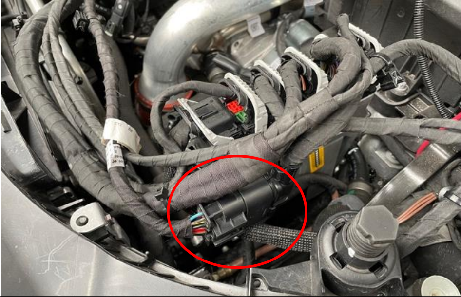
17. Position the terminal around the side of the ECU as shown.
