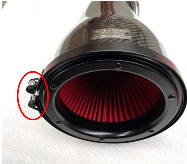
28. Make sure the large clamp around the housing has the bolt on this side as shown. If not, please loosen the clamp and rotate it.
