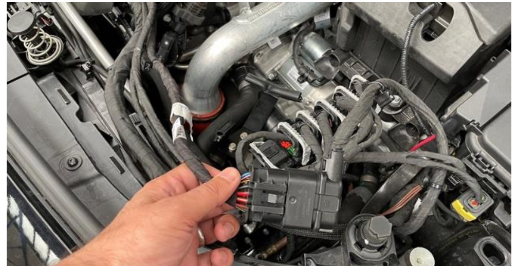
16. Reroute the terminal which was unclipped in step 7. Place the ECU as shown with the plugs facing upwards. See next step for the reroute position.
