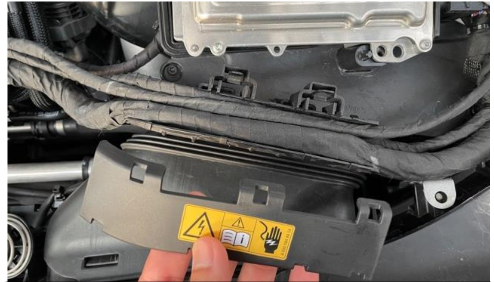
2. Remove the cover of the plastic box holding the wiring loom on the duct. Also remove the zip ties on the inside which secure the loom.
