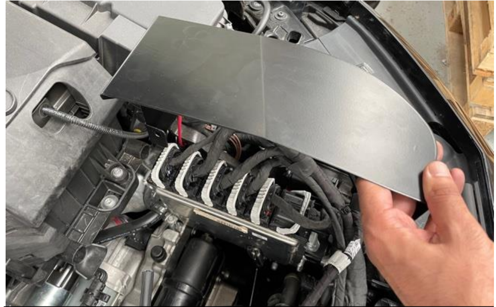
18. Take the cover panel and place it on top of the ECU. See next steps for positioning.
