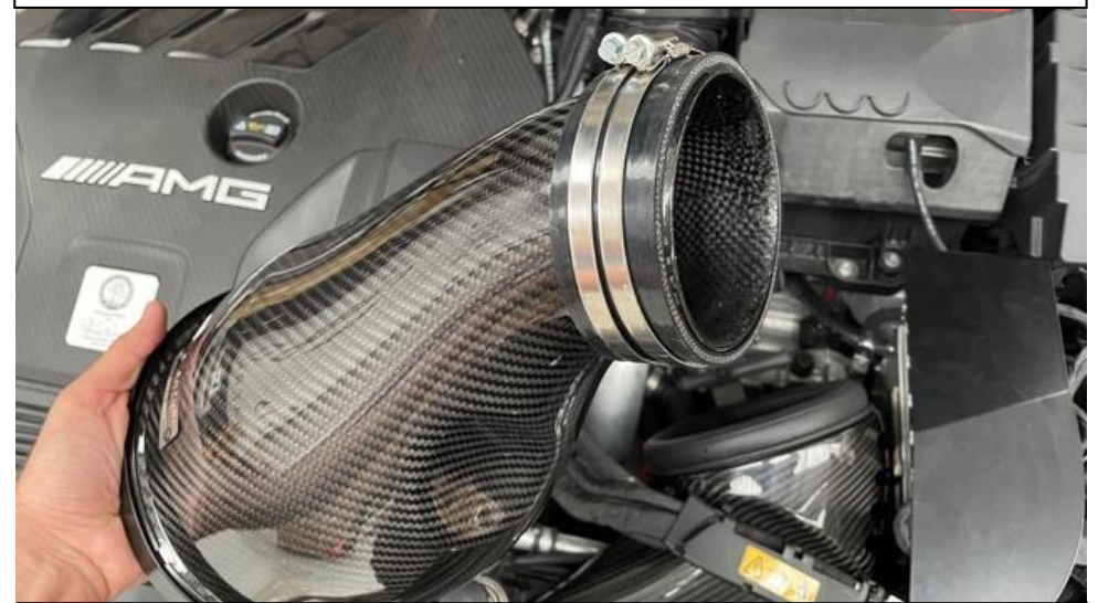
27B. Take the carbon filter housing and push the silicon coupler all the way onto it. Use a little lubrication inside the silicon to make this easier. The silicon should be level with the carbon.
