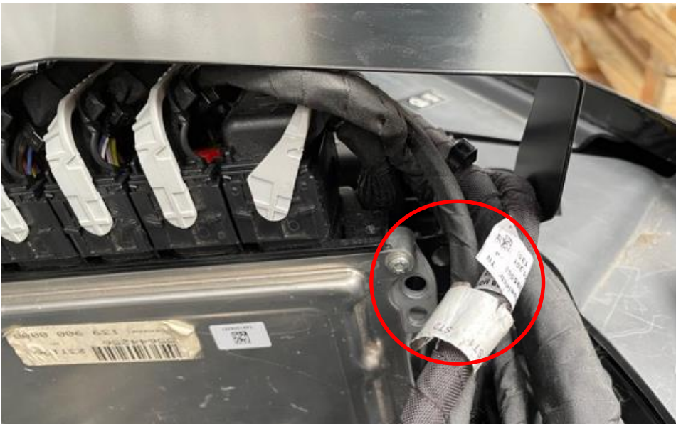
19. Route the tab of the cover under the wiring and position is behind the tab on the ECU as circled.
