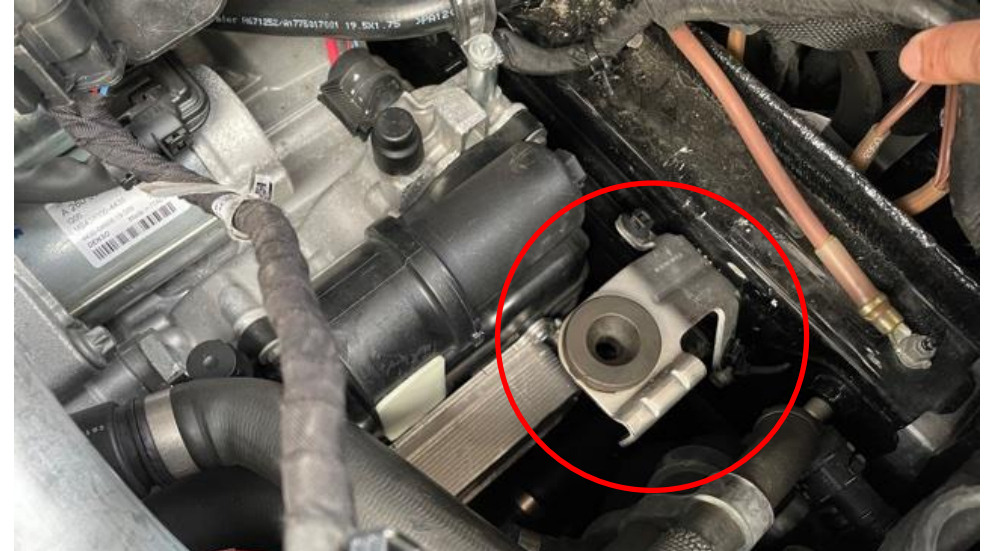
10. This bracket is held in place with 2 x Torx screws. Retain these screws for later.
