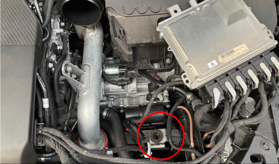
9. Now remove the bracket circled – next step shows a close up.
