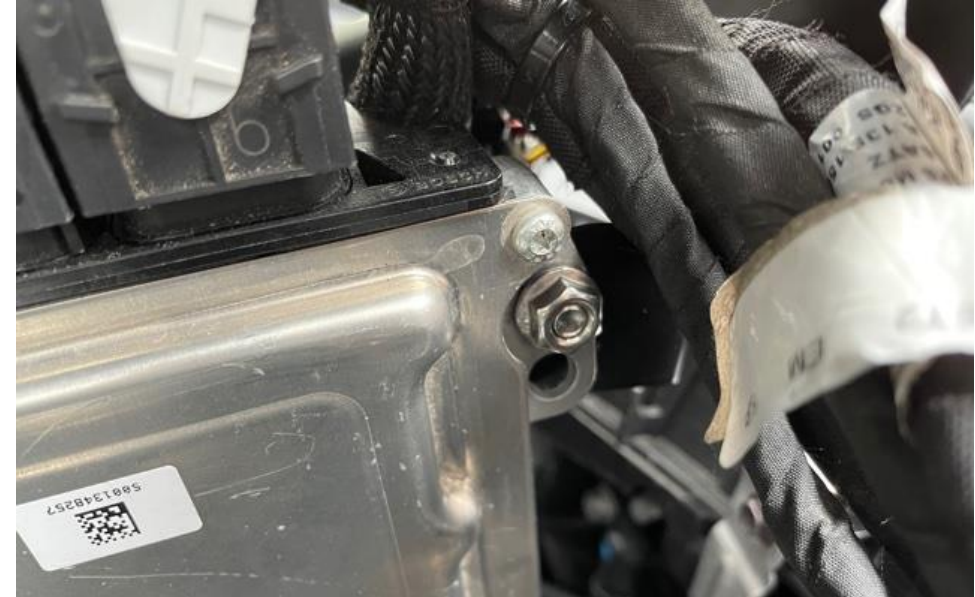
20. Secure this side with an M6 nut and M6 Bolt as shown. Use the upper hole on the ECU tab.
