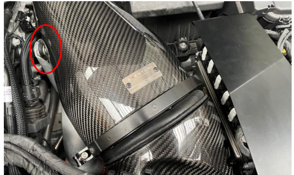
31. Adjust the position of the front so that it sits squarely against the duct rubber seal. Make sure the housing is rotated for clearance with the circled bolt – see next step for close-up.
