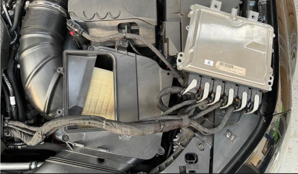
5. Carefully move the ECU away from the airbox.
