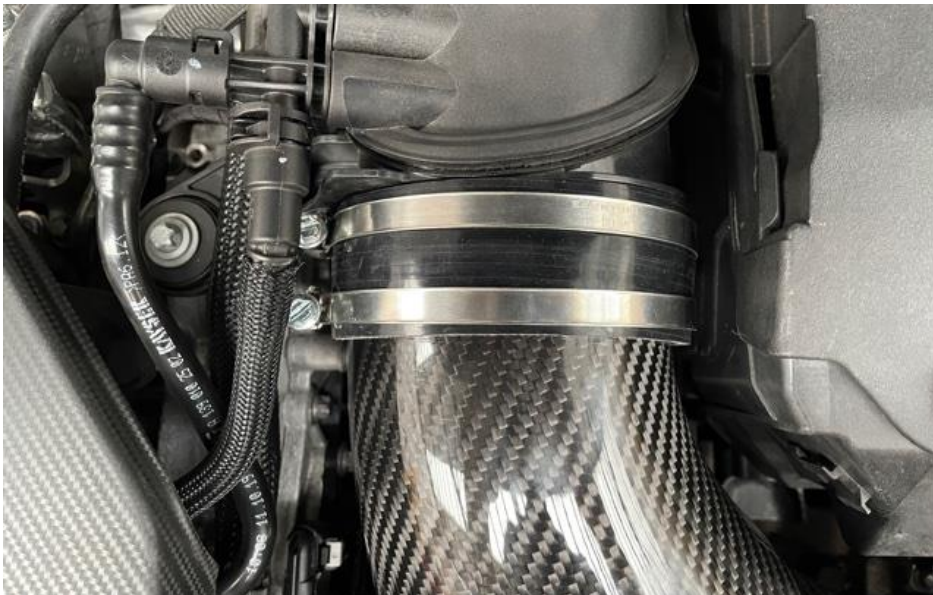
30. Push the silicon onto the turbo inlet – don't tighten the clamps yet.
