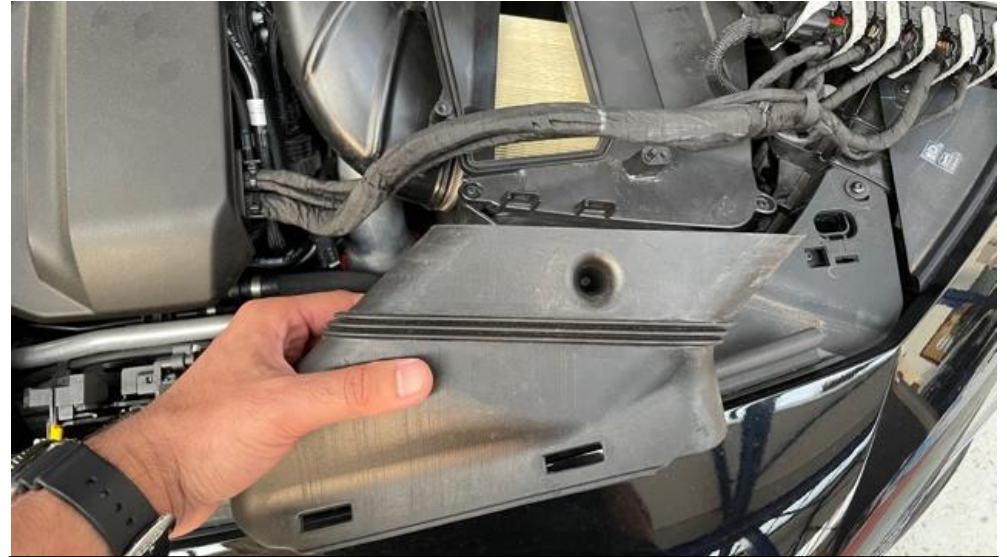
6. Remove the duct by pushing it into the airbox and then lifting it away.
