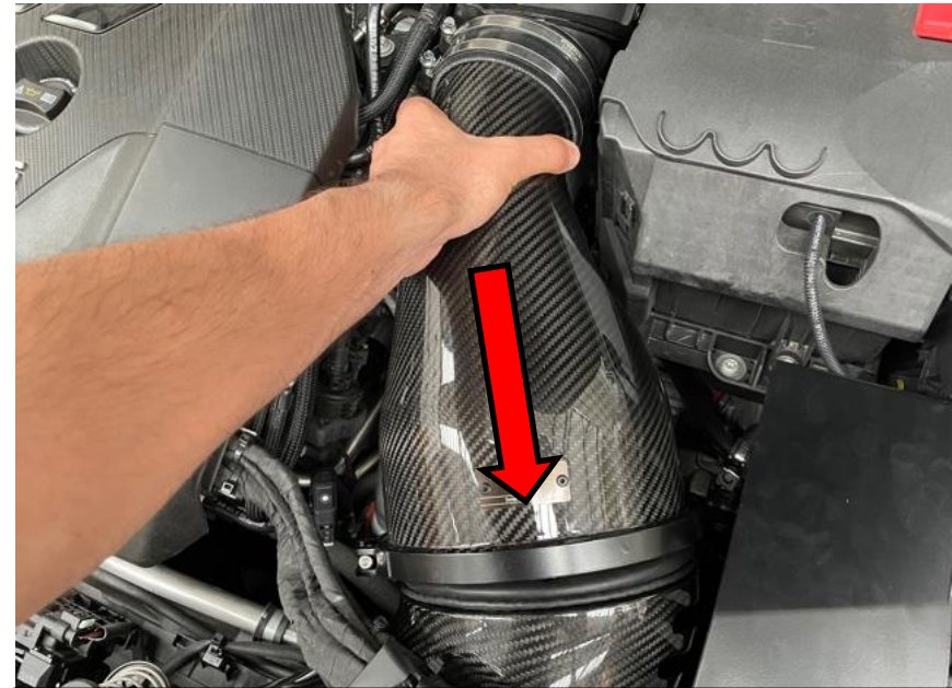
33. Pull the housing forward to compress the rubber seal on the duct. While applying pressure – tighten the clamps around the silicon.
