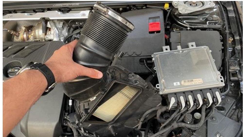
8. Loosen the hose clamp around the intake tube and now the airbox can be removed. It is held in place with a rubber bush at the base and 2 rubber inserts at the back of the airbox in the battery enclosure.
