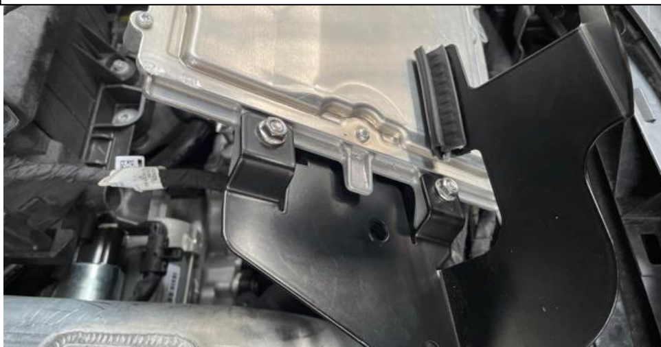
15. Secure with 2 x M6 nuts and 2 x M5x12 bolts.
