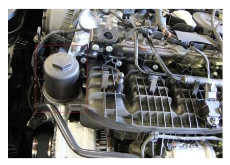
Step 2: Remove factory oil filter housing using 32mm socket. Remove oil filter. Carefully remove the filter cage by pushing it to the side of housing. Transfer oil filter cage to CTS housing, clip into the bottom. Transfer o-ring. Reinstall on vehicle, tighten to 25Nm.
