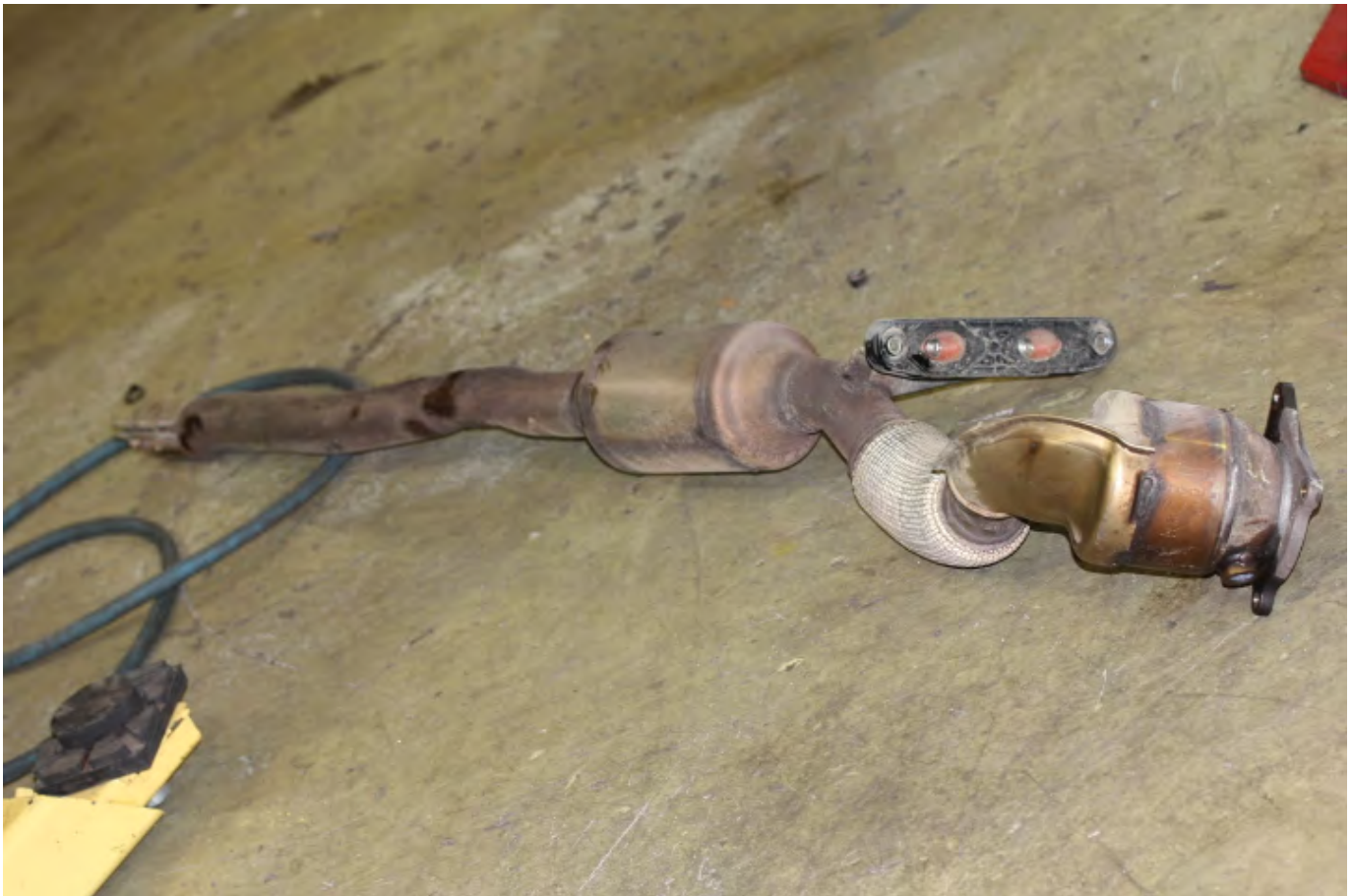
Step 13 - Transfer hanger to new downpipe
