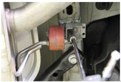
STEP 4. REMOVE HANGERS FROM FACTORY EXHAUST AND TRANSFER THEM TO CTS EXHAUST.
