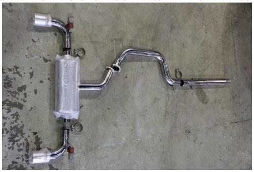
**STEP 5.** INSTALL CTS EXHAUST IN THE CAR, STARTING FROM FRONT AND WORKING TO THE BACK. ATTACH ALL HANGERS. INSTALL GASKET AT THE FLANGE. DO NOT TIGHTEN CLAMPS AND FLANGE BOLTS AT THIS TIME, JUST MAKE THEM SNUG. REINSTALL CROSS BRACE.
