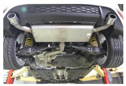
**STEP 2.** Remove 4x 13mm nuts and rear cross brace. Remove factory clamp between downpipe and catback. Remove center exhaust hanger.
