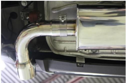
**STEP 6.** CHECK FOR FITMENT AND PERFORM ADJUSTMENTS. THE BEST WAY IS TO WORK FROM BACK TO FRONT IN THIS ORDER: TIPS->MIDDLE CLAMP->FLANGE BOLTS.
