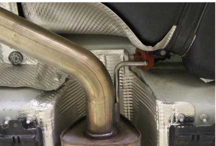
**STEP 3.** REMOVE LEFT AND RIGHT HANGERS (2x 13MM BOLTS) AND REMOVE FACTORY EXHAUST
