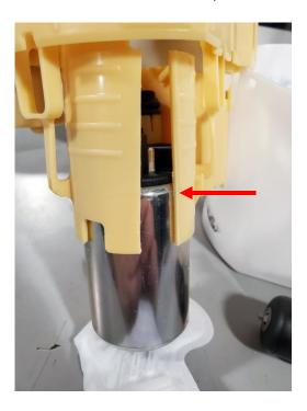
6 – Carefully remove the OEM connector guide, and the small arms that limit how high the pump can insert, this will allow the DW440 pump to orientate itself correctly and allow full engagement of the o-rings to seal.
