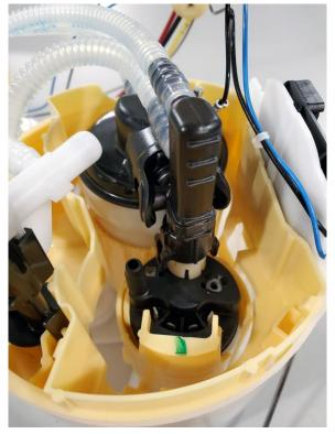
10 – The DW440 Brushless pump wiring is different from the OEM pump wiring. There are two ways to correct this. We have supplied a pigtail and fuel safe heat shrink butt connectors if you would like to cut and crimp the correct connector on or the OEM Toyota connector can be re-pinned easily and will connect to the DW pump.
