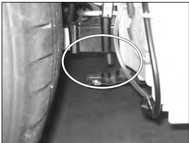
Cut the circled portion so Hose Assy ① does not come in contact with.
