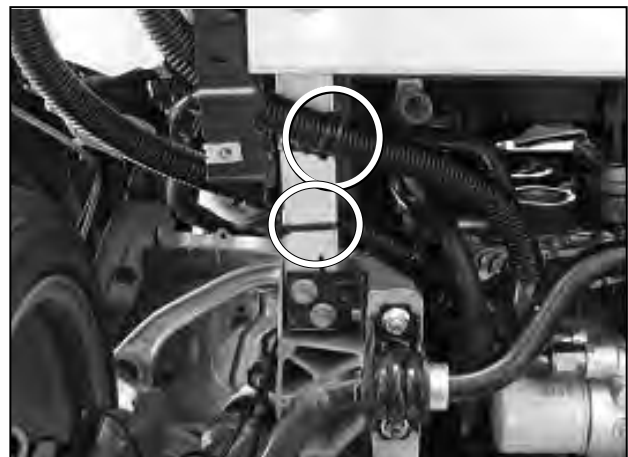
Secure the Hose Assy to the side member. ▪ Tie Wrap (M) (x2) ▪ Tie Wrap (L) (x2)
